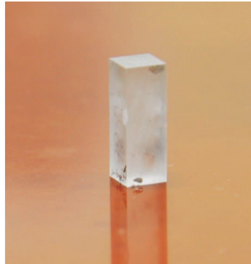
Fig. 1 Picture of the 15 mm long 9.8 at% Yb:YAG ceramics block.
