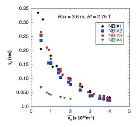
Fig. 4 Measured  $\tau_n$  as a function of line-averaged electron density for the plasma with  $R_{ax} = 3.6$  m and  $B_t = 2.75$  T.
