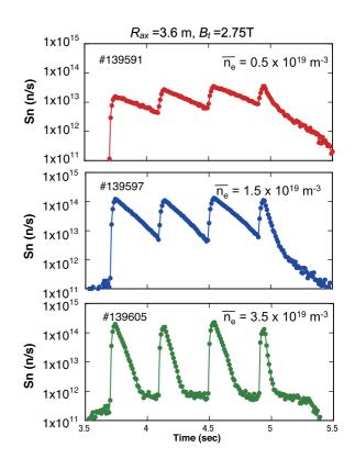
Fig. 3 Time histories of the neutron emission rate at the NB blip experiments with different electron density.
