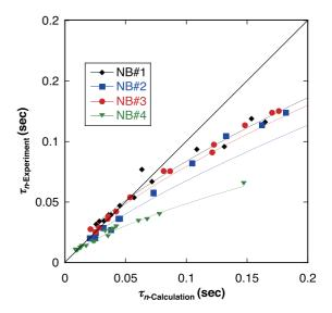
Fig. 6 Comparison of calculated and measured  $\tau_n$  for the plasma with  $R_{ax} = 3.6$  m and  $B_t = 2.75$  T.
