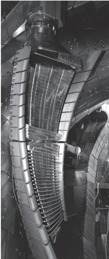
Fig. 1 Photo of the PA antenna without FS (upper) and with FS (lower).
