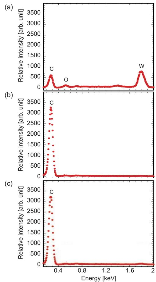
Fig. 3 EDX spectra of (a) W1, (b) W3, and (c) W5.
