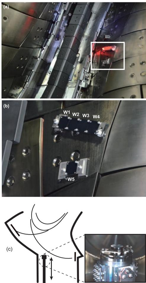
Fig. 1 (a, b) Pictures of the samples equipped in the LHD vacuum vessel and (c) a schematic of the configuration of the sample holder in LHD.
