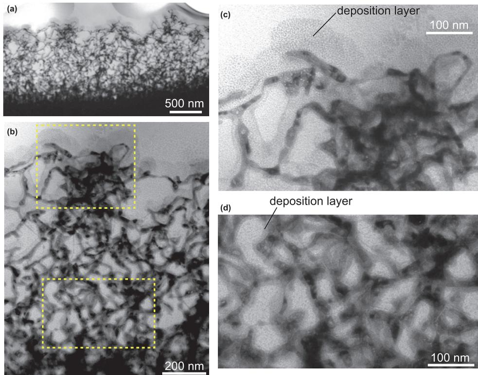
Fig. 9 TEM micrographs of W7 in different scales. (c) and (d) are the top part and deep part of the structures.
