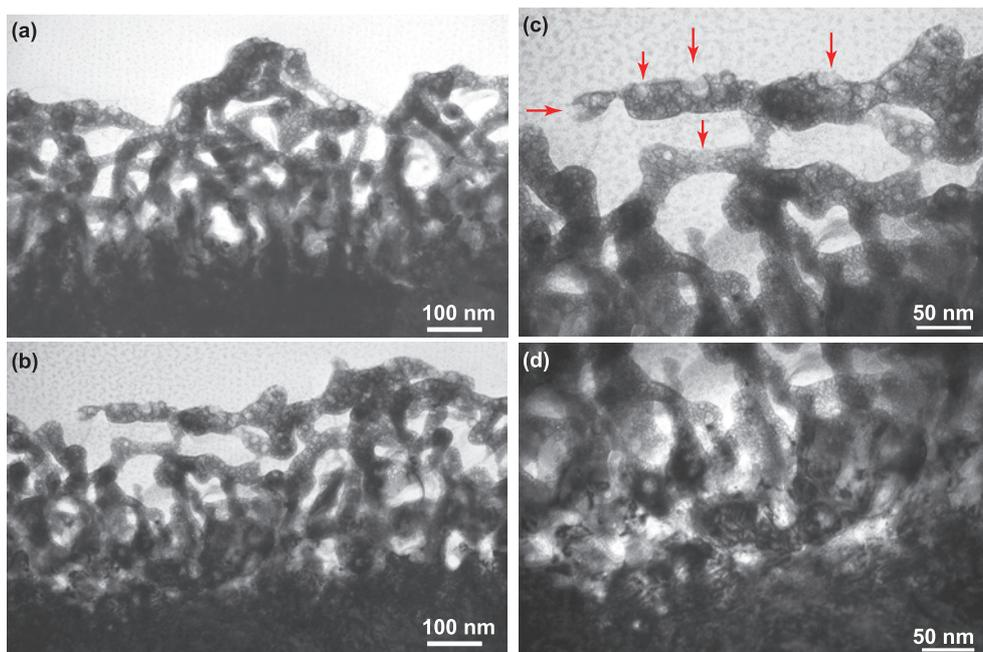
Fig. 5 TEM micrographs of the cross section of W1. (a) and (b) are from the same sample but at different positions. (c) and (d) show the head part and bottom part of the structures, respectively, in a larger magnification.
