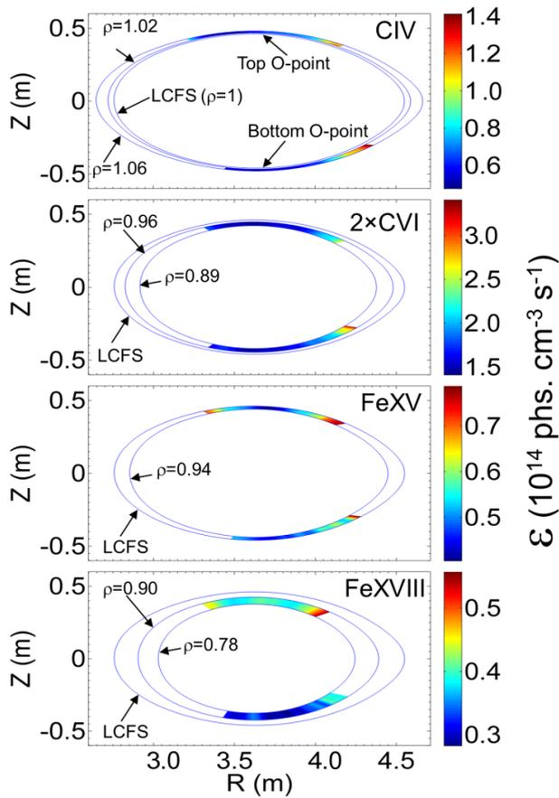
Fig. 6 Poloidal distributions of (a) CIV, (b) CIV, (c) FeXV and (d) FeXVIII at horizontally elongated plasma cross-sections. The measure of the emissivity is represented by different colors.
