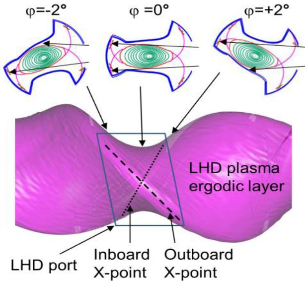
Fig. 1 Horizontal view of LHD ergodic layer and poloidal plasma cross-sections at three different toroidal angles  $\varphi = -2^\circ, 0^\circ$  and  $+2^\circ$ .
