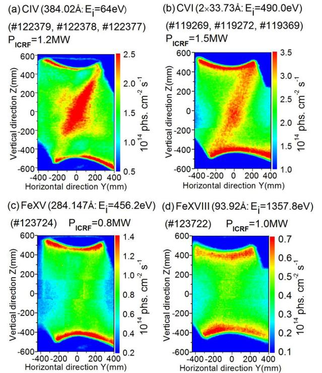
Fig. 2 2-D distributions of (a) CIV, (b) CVI, (c) FeXV and (d) FeXVIII at  $R_{\text{ax}} = 3.60$  m. The shot numbers and ICRF power are indicated in each distribution.
