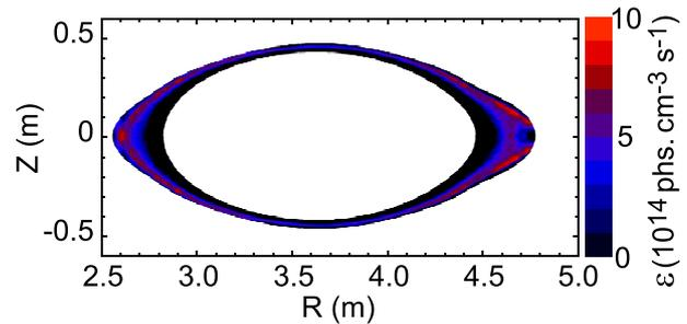
Fig. 8 Simulation of emissivity distribution of CIV ( $312.4 \text{ \AA}$ ) using EMC3-EIRINE code under similar conditions as the experiment.
