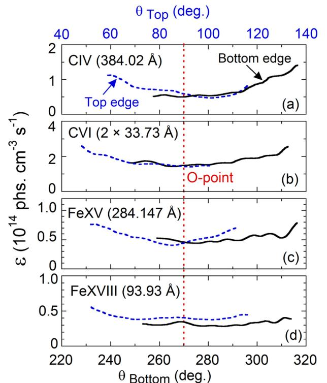
Fig. 5 Poloidal distributions of (a) CIV, (b) CVI, (c) FeXV and (d) FeXVIII as a function of poloidal angles  $\theta_{\text{Top}}$  and  $\theta_{\text{Bottom}}$ .
