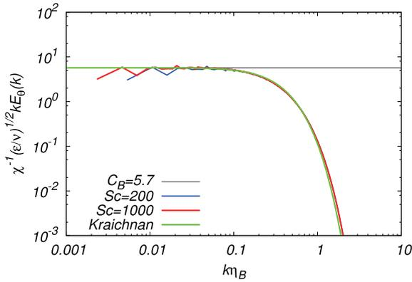
Fig. 5 Comparison of compensated three dimensional scalar variance spectrum at  $Sc = 1000$ . The Kraichnan spectrum is computed with  $C_B = 5.7$ .
