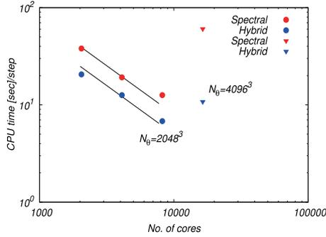
Fig. 3 Comparison of CPU time for spectral and hybrid codes at  $Sc = 1000$  measured on Plasma Simulator. In the spectral computation, the numbers of grid points of the velocity and scalar are  $N_v = N_\theta = 2048^3$  for red circle and  $N_v = N_\theta = 4096^3$  for red triangle. In the hybrid computation,  $N_\theta = 2048^3$  for blue circle and  $N_\theta = 4096^3$  for blue triangle, and  $N_v = 256^3$  for two cases.
