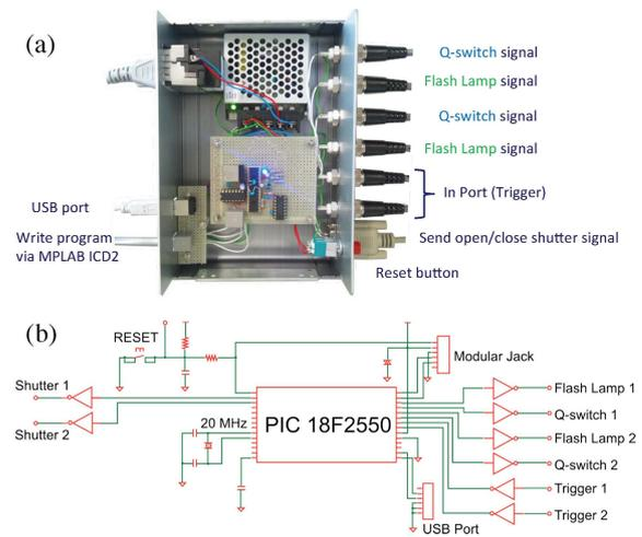
Fig. 1 (a) Top view of the timing controller and (b) its circuit diagram.
