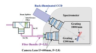
Fig. 1 Sketch of diffractive beam splitter, optics and the spectrometer.
