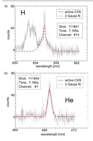
Fig. 6 The background subtracted spectra are fitted by two Gauss functions. a): Hydrogen spectrum. b): Helium spectrum.
