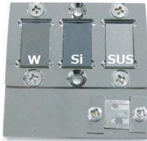
Fig. 1 A set of fresh specimens on the material probe.
