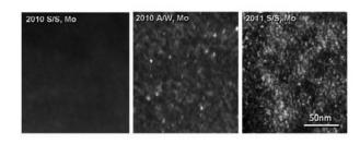
Fig.2 Formation of dislocation loops in Mo placed at equator part in the campaigns of 2010S/S, 2010A/W and 2011S/S.
