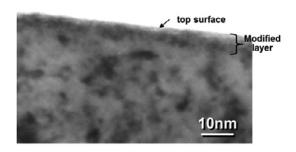
Fig.1 Cross-sectional TEM images of Mo exposed to 2011S/S plasmas at equator part of the inner wall.
