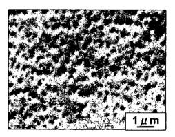
Fig. 2 SEM image of tungsten surface exposed to divertor plasma of hydrogen discharge
