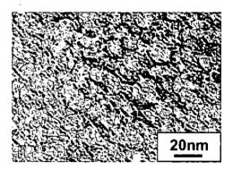
Fig. 1 TEM image of tungsten exposed to helium discharge cleaning
