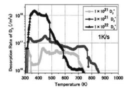
Fig.2 Thermal desorption of injected D from the 316LSS coupons covered with 21nm-thick deposition. Corresponds to 2012AW-P16-E
