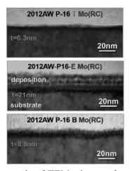
Fig. 1 Cross-sectional TEM micrographs showing impurity deposition on Mo coupons place at top, equator and bottom wall.
