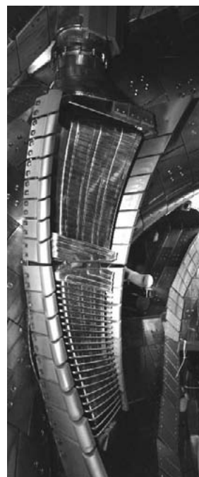
Fig. 1 ICRF antennas with and without Faraday shield in LHD in 2013
