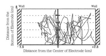
Fig. 1 An example of trace of the foreign substance. Under 60 Hz, in air.
