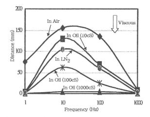
Fig. 2 Motion of a foreign substance as a function of frequency of the applied voltage.
