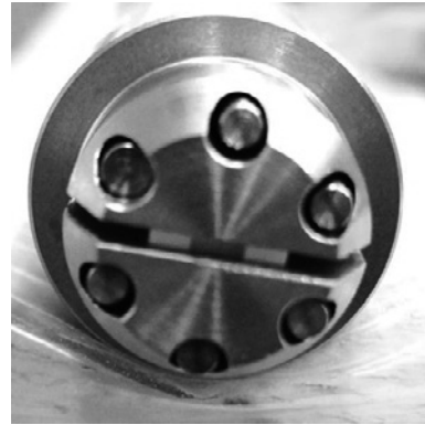
Fig. 1: A picture of the probe head. The arrangement of electrodes can be seen.
