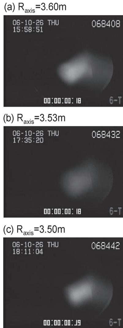
Fig. 1. Tangential view of CCD camera. The shift of initial plasma can be seen.
