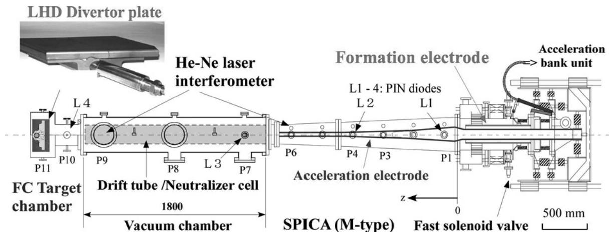
Fig.1 Schematic view of the pulse heat flux material test system by using the SPICA CT injector.
