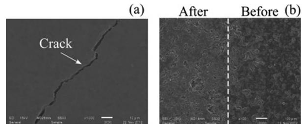
Fig. 2. SEM images show the surface morphology of (a) W after pulsed plasma irradiation, (b) graphite divertor plate before and after irradiation.
