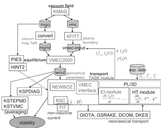
Fig.1 Module structure for the integrated transport simulation
