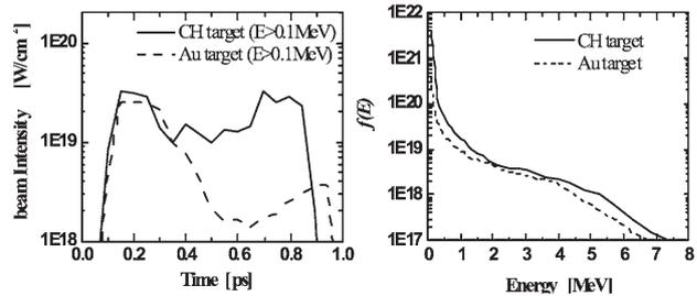
Fig.1 Results of 1D PIC simulations; the left one is the temporal evolution of fast electron beam intensity and the right one the time integrated fast electron spectra for Au and CH cone
