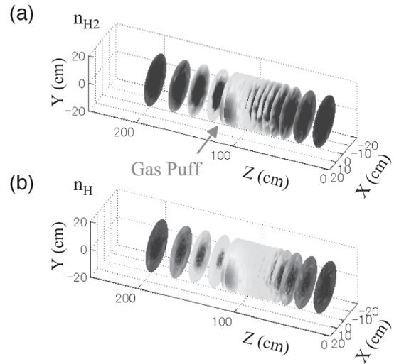
Fig. 2. Predicted atomic (a) and molecular (b) hydrogen density obtained by the DEGAS simulation.
