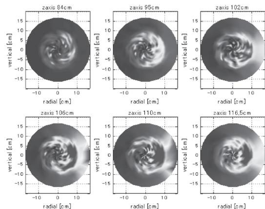
Fig. 3 Cross-section view of the H $\alpha$  emissivity calculated from DEGAS.
