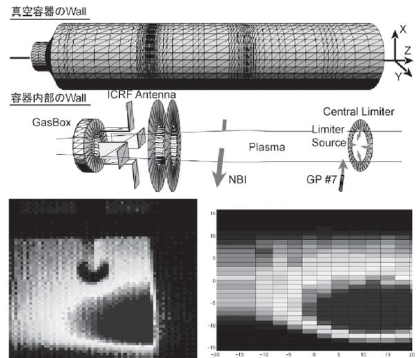
Fig. 1. Upper: Fully 3-dimensional mesh model of the GAMMA 10 central-cell, Lower left: 2-dimensional image in GPI experiment in the central-cell. Lower right: Simulation result of the GPI experiment.
