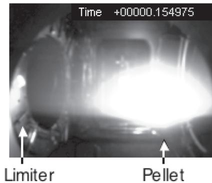
Fig. 2. Ablation light of hydrogen pellet in the central-cell measured with a high-speed camera.
