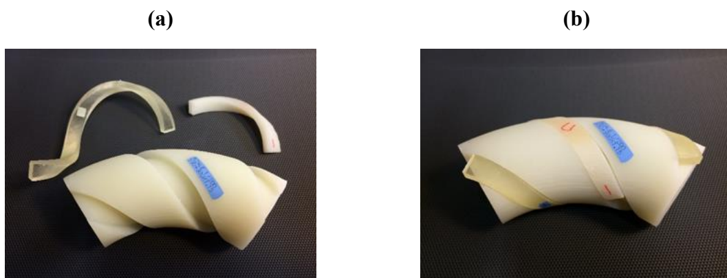
Figure 2.4.4.6 Confirmation of HTS joint-winding by 3-D printing models.
