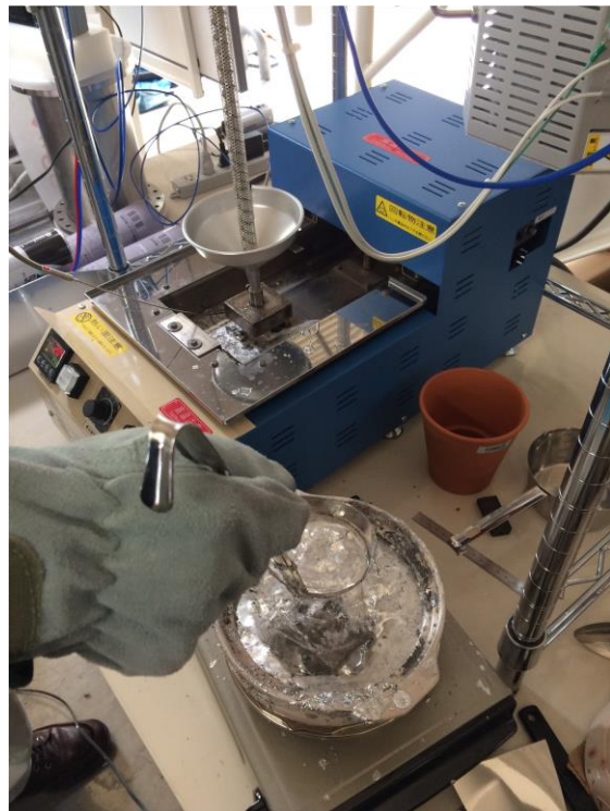
Figure 3.5.6.7 The solder jet bath (Tsunatori Electric Manufacturing Co., Ltd, NTD-01).
