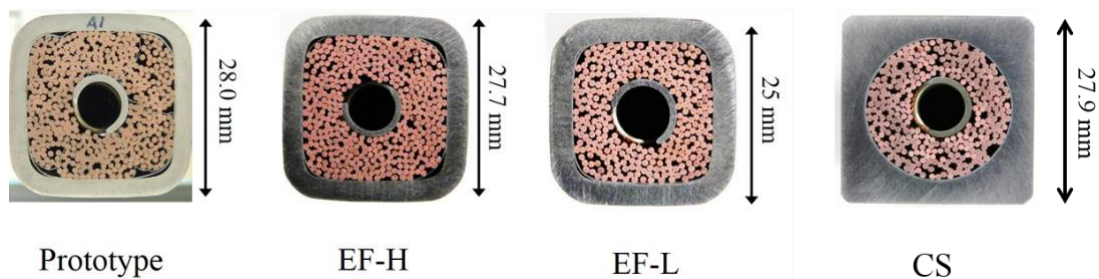
Figure 3.1.1.5 Photographs of the CIC conductors used for the EF and CS coils of JT-60SA.
