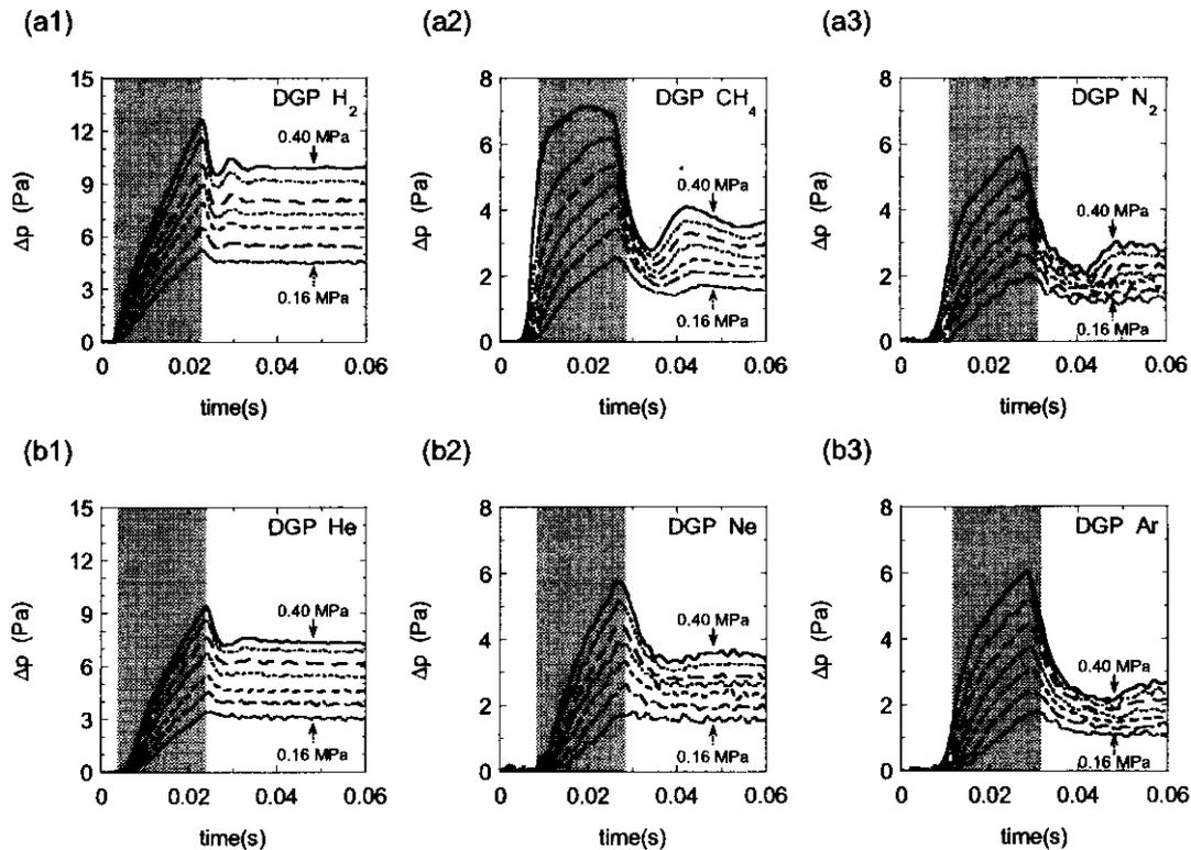
Fig. 4. Experimental results of the gas flow velocity measurement with the DGP configuration; (a1) hydrogen, (a2) methane, (a3) nitrogen, (b1) helium, (b2) neon, and (b3) argon. Shaded region denotes the time-shifted gas puff pulse width (see text). The absolute primary pressure of the piezo-valve is increased from 0.16 to 0.40 MPa, with an increment of 0.04 MPa. In each pressure, same experiment is repeated five times and shown in the figure is the averaged waveform.
