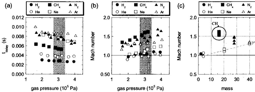
Fig. 5. (a) Measured  $t_{\text{delay}}$  and (b) the Mach number,  $M$ , as a function of the absolute primary pressure of the piezo-valve. (c)  $M$  versus the mass number of the working gas molecule, where the primary pressure is 0.27 – 0.34 MPa (corresponds to the shaded region in (a) and (b)).
