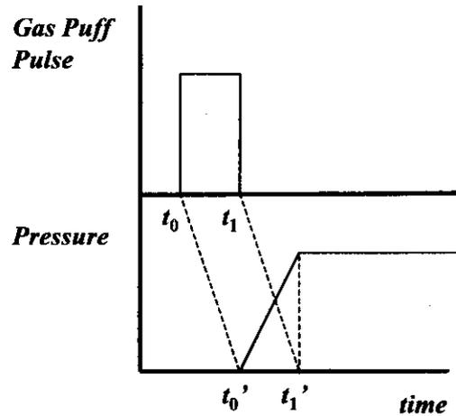
Fig. 3. Expected waveform of the pressure signal.
