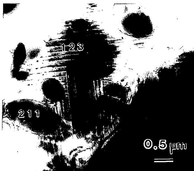
Fig.10.2-3 Transmission electron micrograph of Y-Ba-Cu-O fabricated by the melt process with melt-quenched precursors.
