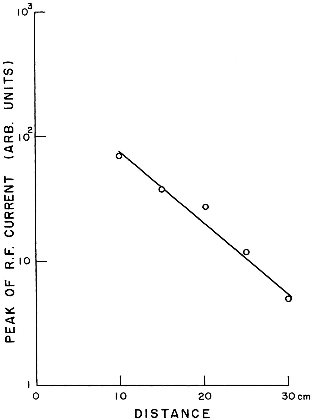
Fig. 6.2. Dependence of the amplitude of the resonance on the distance between the transmitting and the receiving probes. Low density case.
