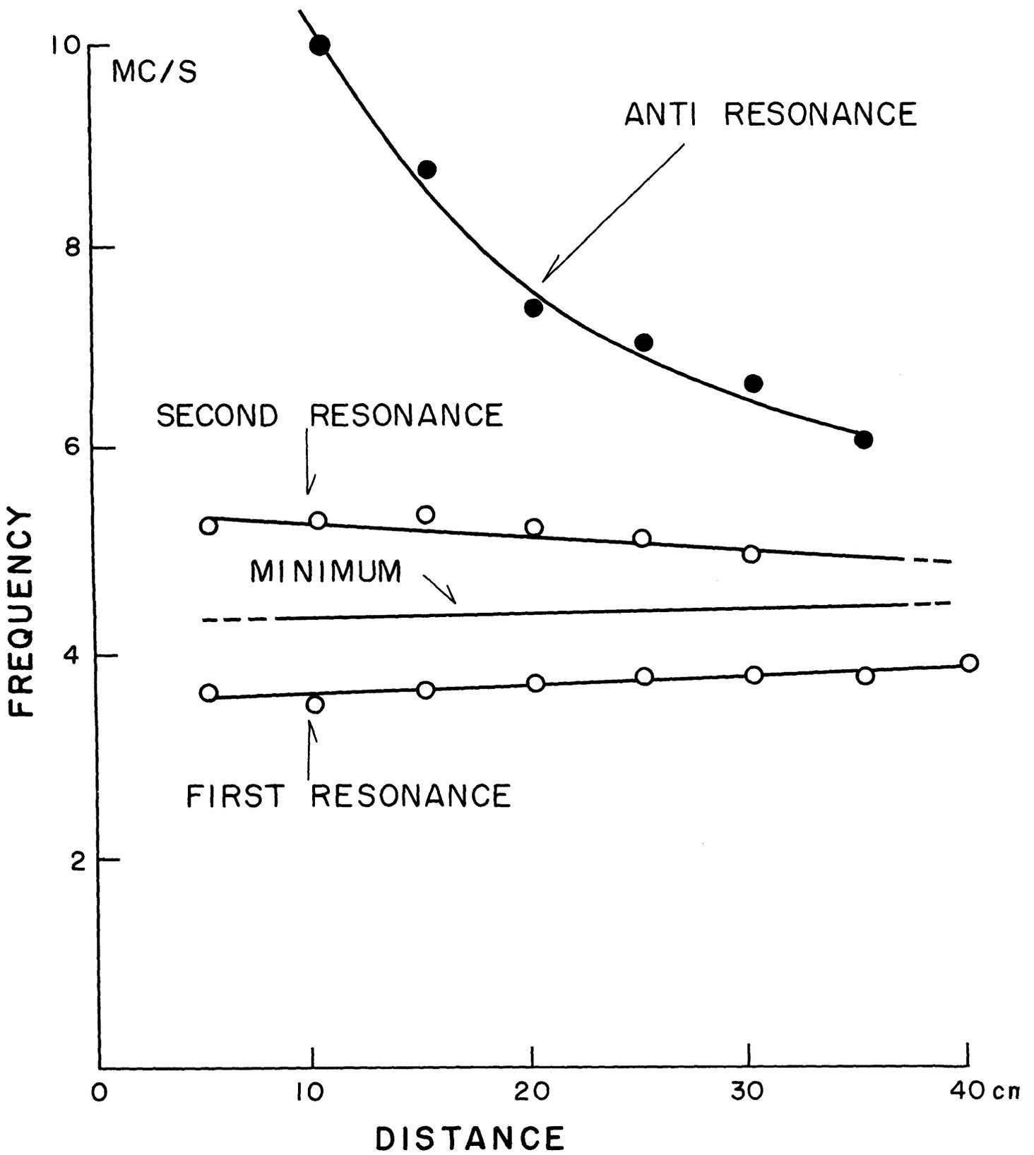
Fig. 5.1. Dependence of the frequency of the resonances and of the minima on the distance between the radial probes. High density case.
