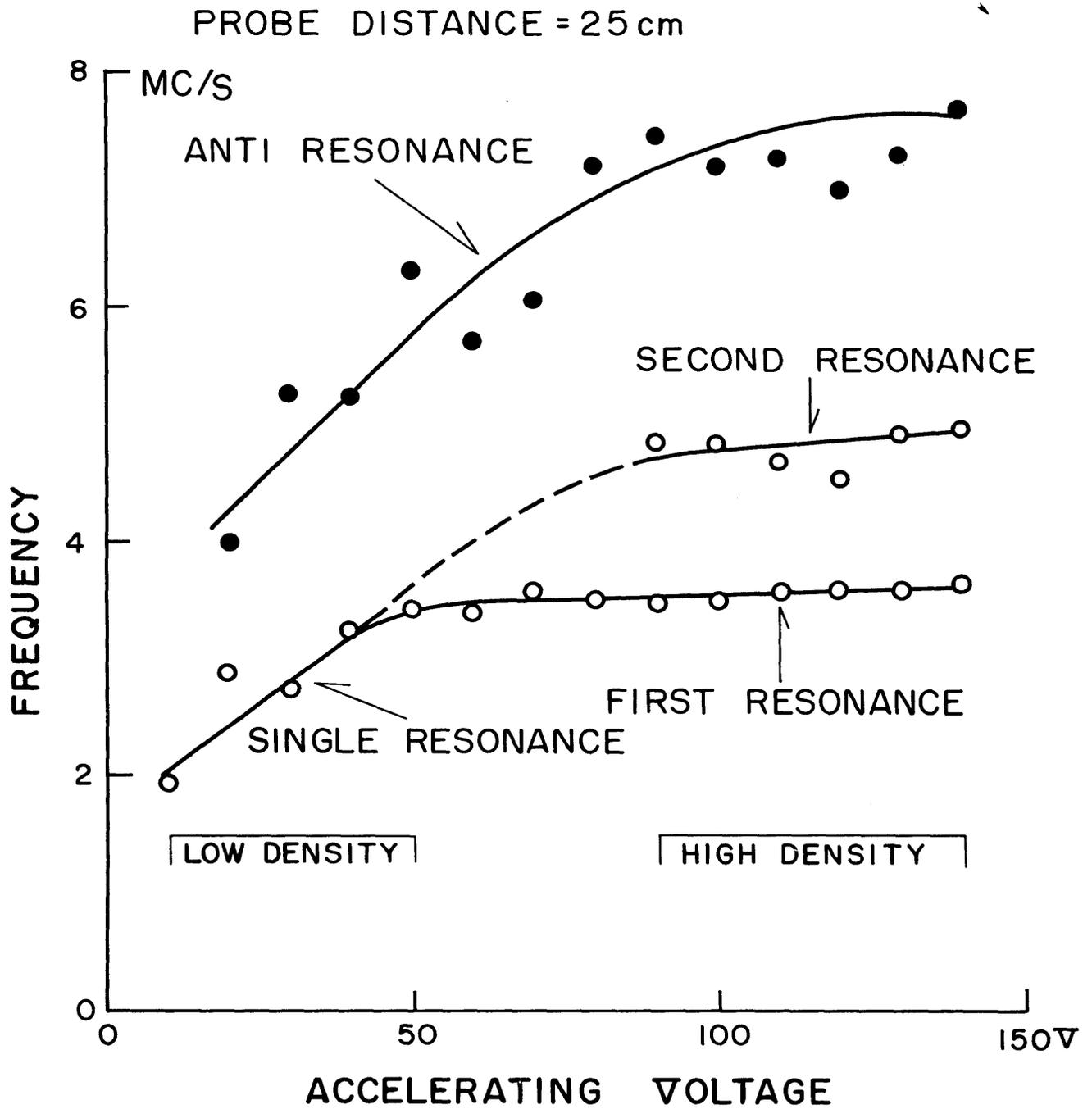
Fig. 7.1. Transition from the low density to the high density case, for growing acceleration voltages. Frequency variation of the resonance, from single to double.
