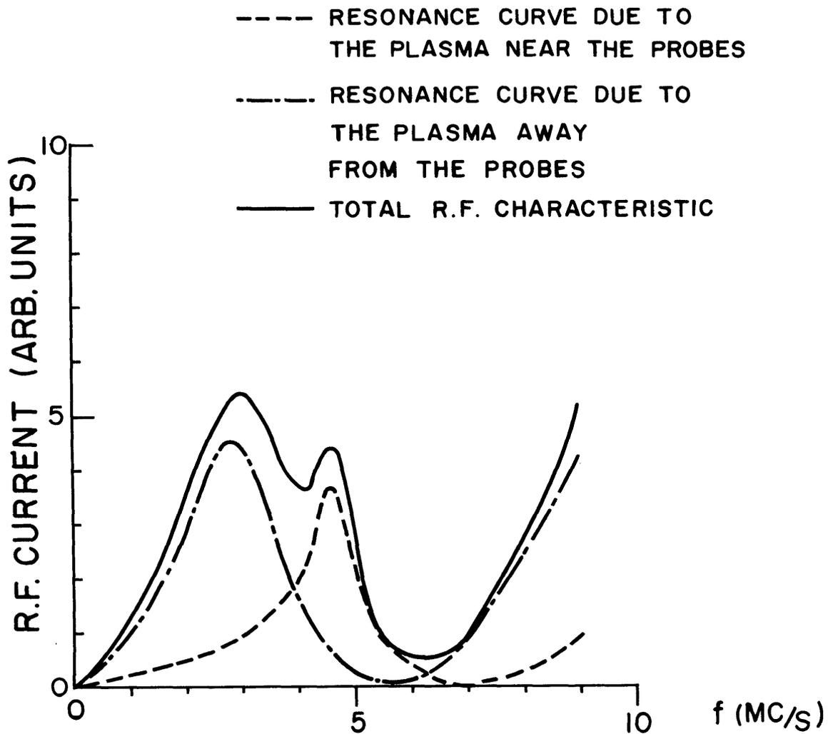
Fig. 8.2. Model explaining the high frequency and the low frequency resonances. Large distances ( $D = 30\text{cm}$ ). Structure of the characteristics.
