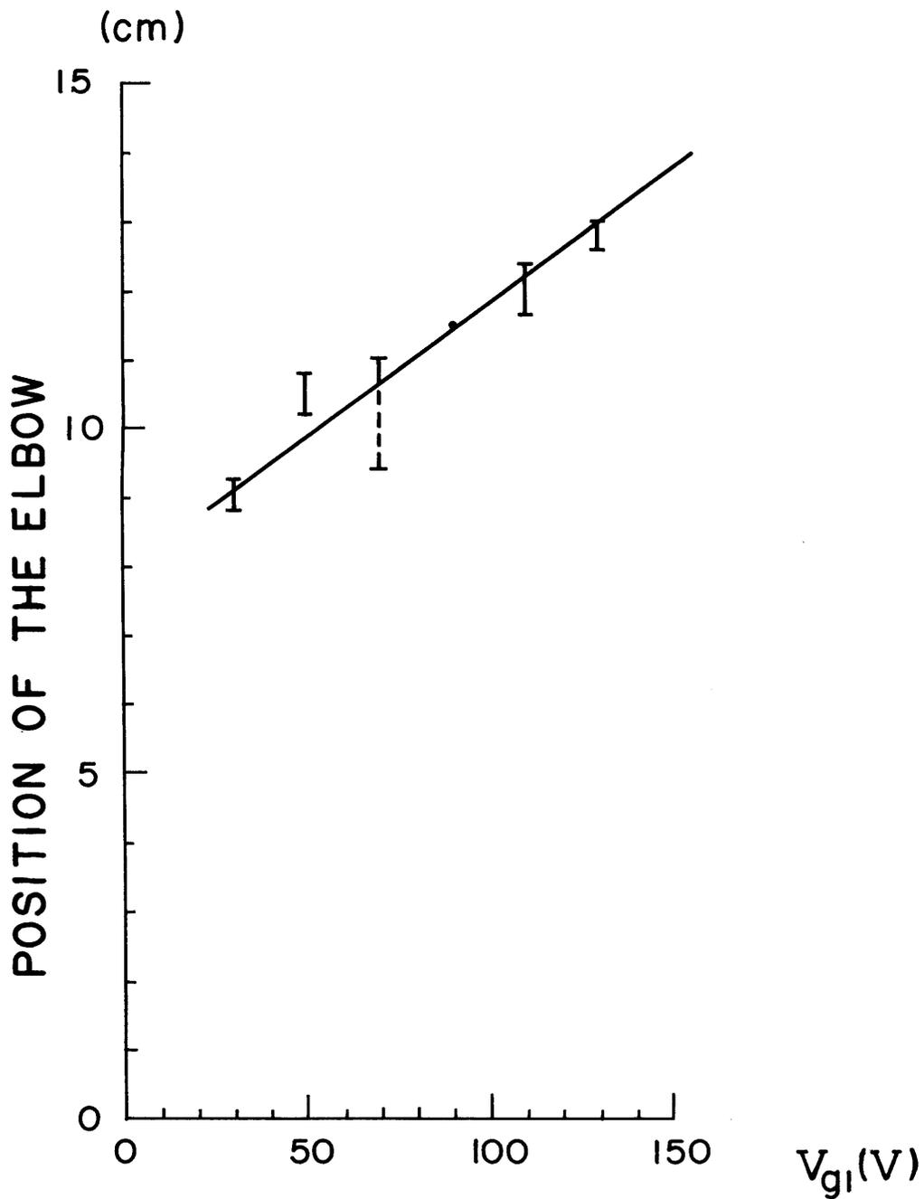
Fig. 3. Position of the elbow, between the internal and the external wings of the radial density profile, versus acceleration voltage.
