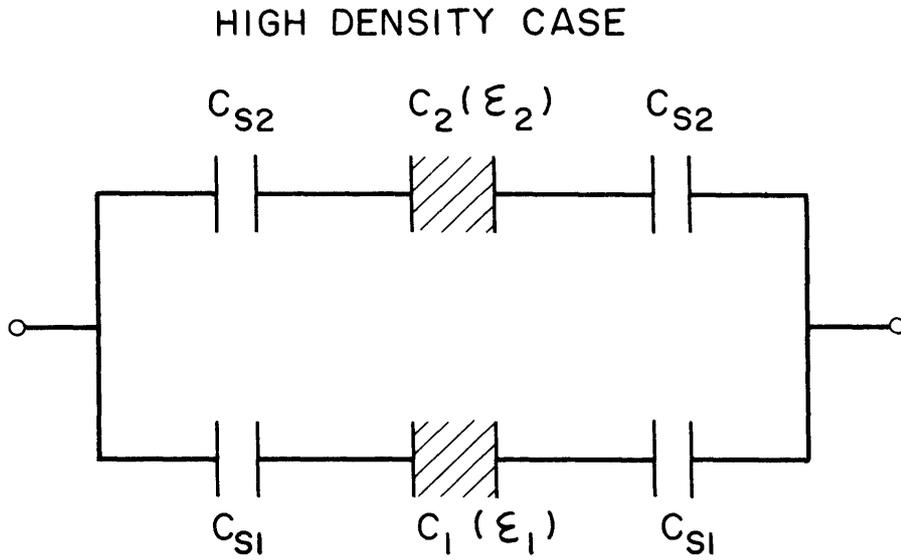
Fig. 8.3. Model explaining the high frequency and the low frequency resonances. Equivalent circuit: high density case.
