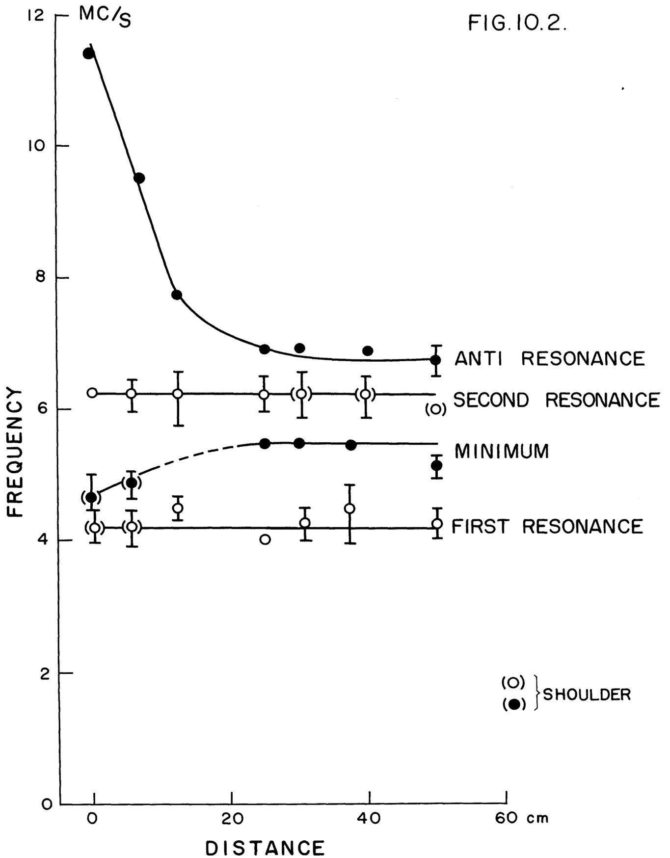
Fig. 10.2. Variation of the frequency of the resonance peaks and of the minima for different axial positions of the receiving probe.
