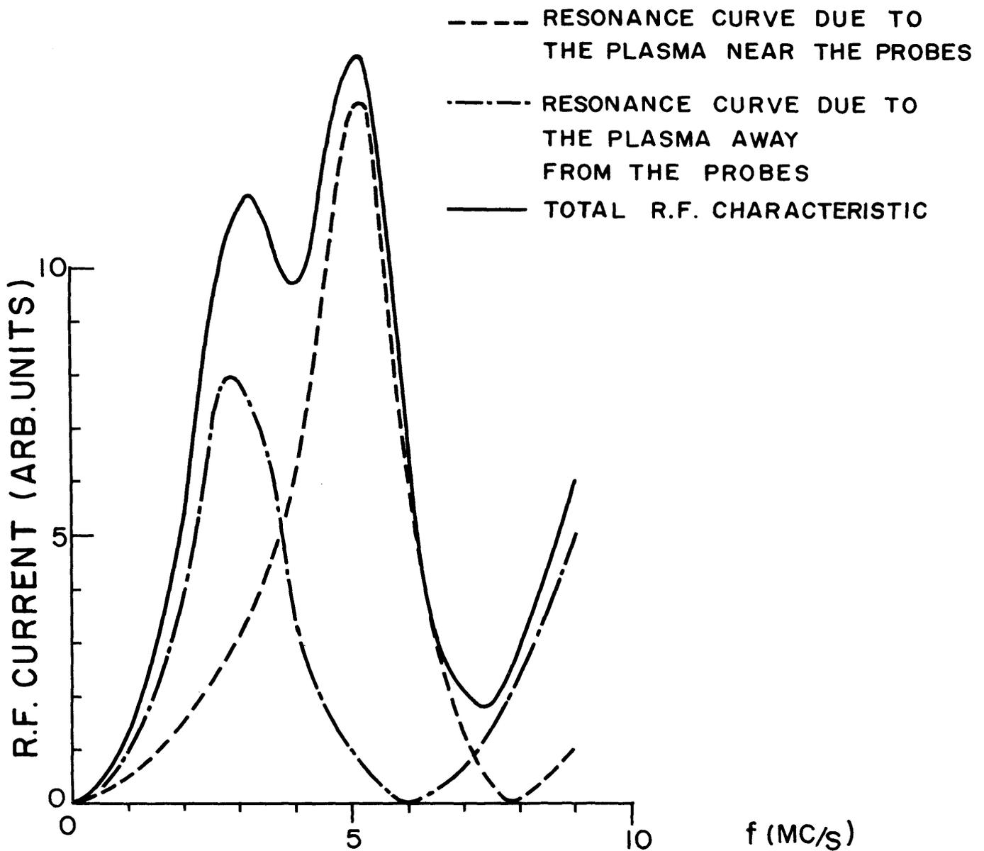
Fig. 8.1. Model explaining the high frequency and the low frequency resonances. Small distances ( $D = 10\text{cm}$ ). Structure of the characteristics.
