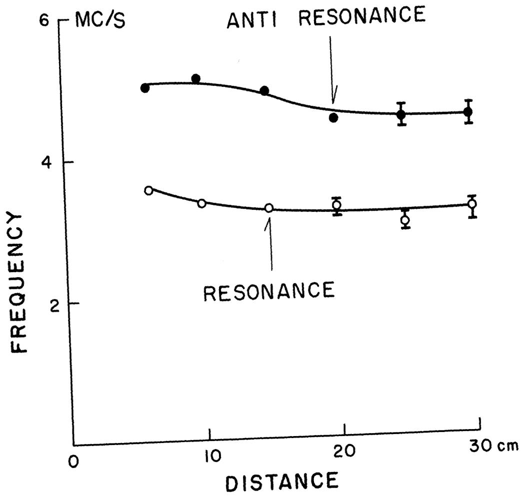
Fig. 9. Dependence of the frequency of the resonance and of the antiresonance, on the distance  $D$  between the probes, for a high density type plasma. The probes are located in the central plane of the metal vessel.
