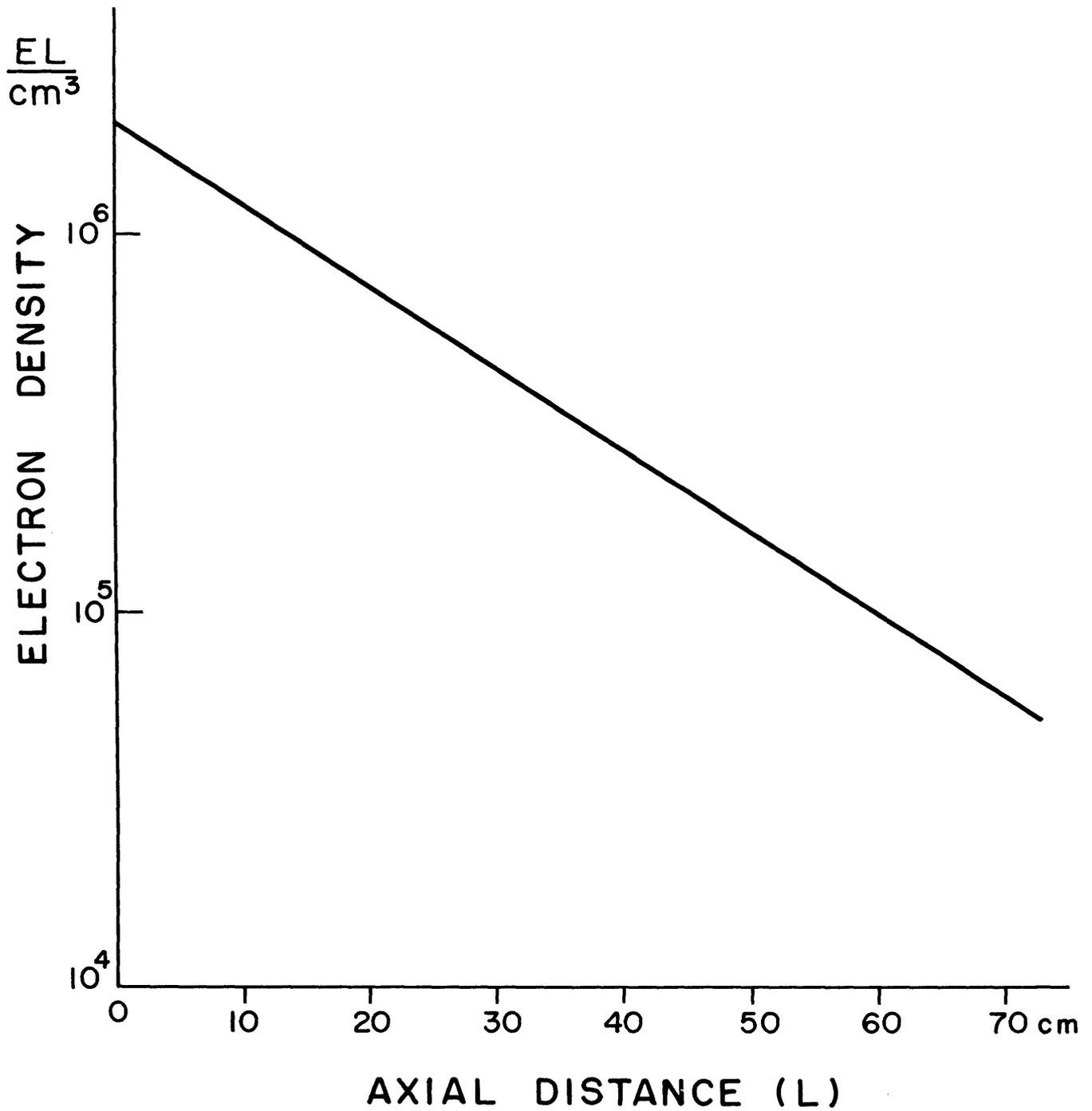
Fig. 10.1. Axial density decay, during the longitudinal r.f. measurements. High density case. The distance L is measured from the plane where the radial probes are located.
