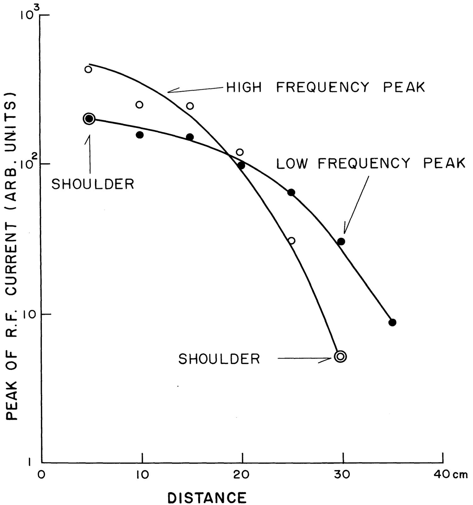
Fig. 5.2. Dependence of the amplitude of the resonances on the distance between the radial probes. High density case.
