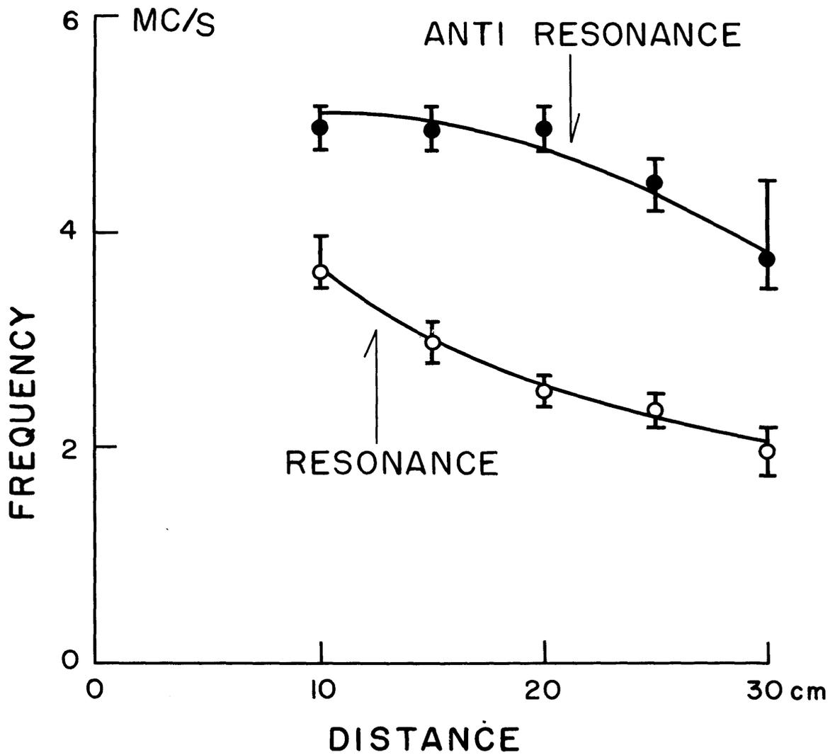
Fig. 6.1. Dependence of the frequency of the resonance and of the antiresonance on the distance between the transmitting and the receiving probes. Low density case.
