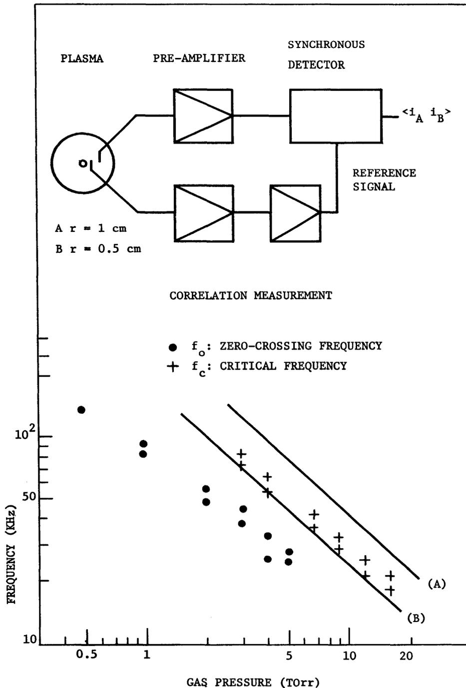
Fig.4 The block diagram for the measurement of the correlation function, and the pressure dependence of  $f_c$  and  $f_o$ . The solid line (a) is calculated from the relation,  $f_c = (1/\pi)D_e r^{-2}$ , with the assumption  $D_e = V_{th} \lambda/3$ , and the curve (b) is calculated by using Einstein relation  $D\tau = r^2 \alpha^2$  in cylindrical dimension ( $\alpha$  is the first root of the Bessel function  $J_0$ ).
