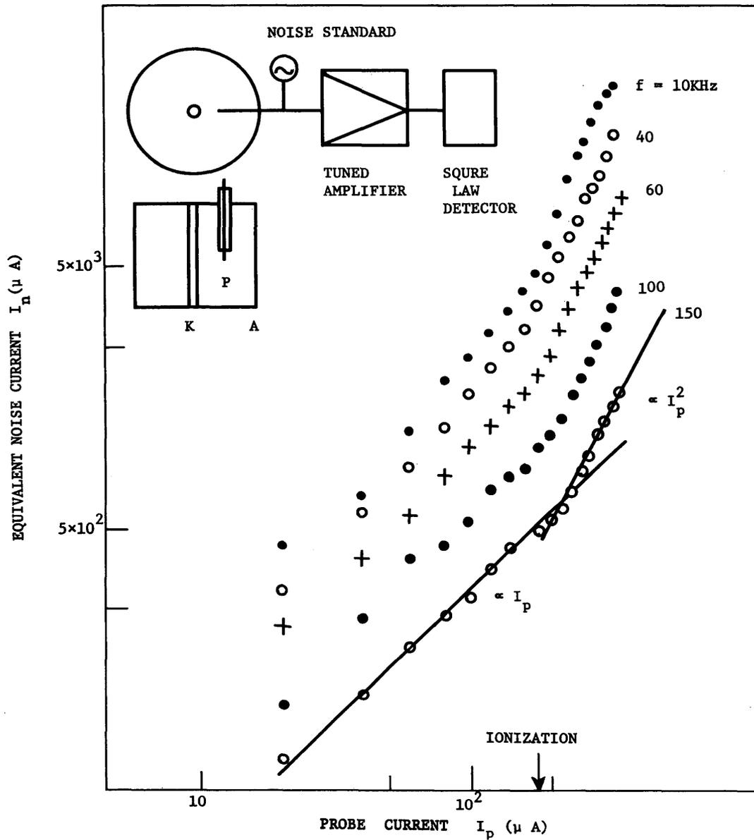
Fig.1 The block diagram of the instrumentation; the structure of the discharge tube and the  $I_p - I_n$  characteristics.
