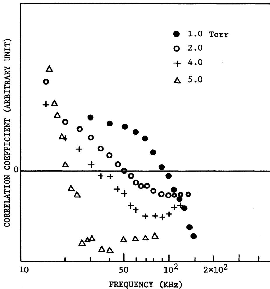
Fig.3 The results of the measurement for  $\langle i_A i_B \rangle$  or  $G(r, r', \omega)$ . As the increase of the gas pressure, zero-crossing frequency becomes lower. The signal was obtained by the probes which were biased to the space potential.
