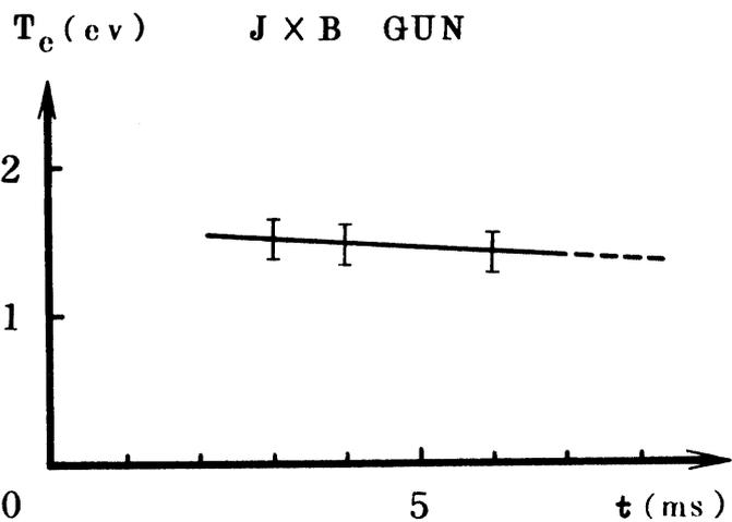
Fig. 5 Typical signal of ion saturation current of the J × B type gun ( 1  $\mu$ A/div, 1 ms/div.). The lower figure shows the time variation of the electron temperature.
