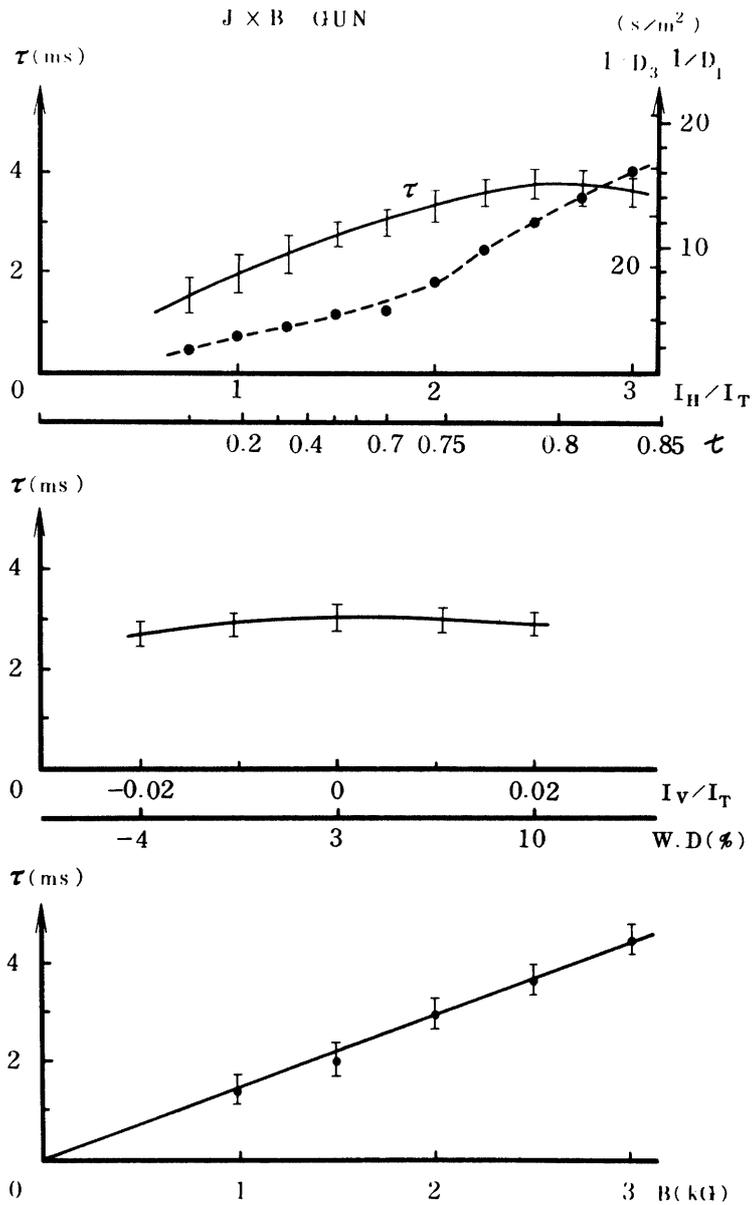
Fig. 6 The dependence of confinement time  $\tau$  on the rotational transform angle and the well depth (W.D.) is shown when the toroidal field is 2 kG. The dependence of  $\tau$  on the magnitude  $B$  of the toroidal field is also shown when the ratio of currents of helical coil to toroidal field coil is 2. The inverse of the diffusion coefficient  $1/D_1$  and  $1/D_3$  are given in the top figure.
