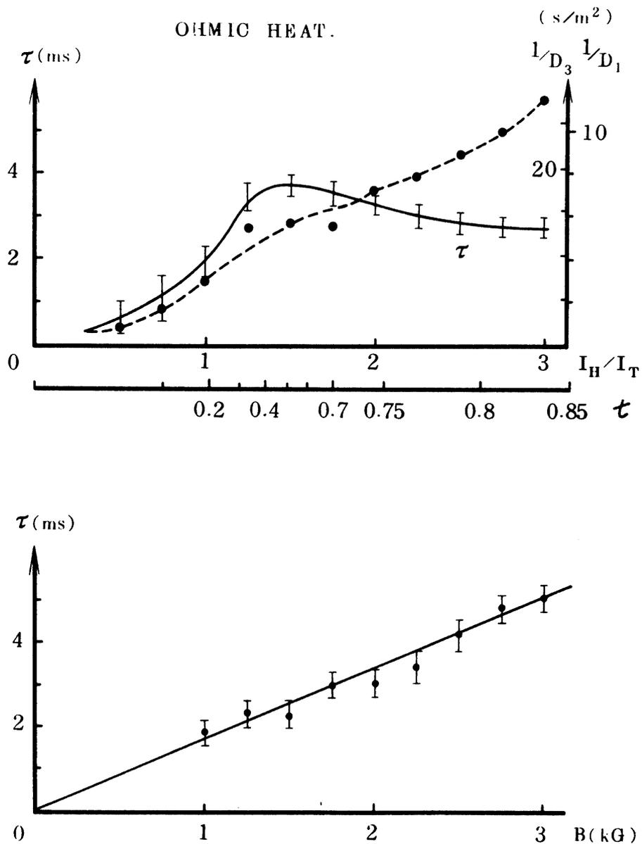
Fig. 9 The upper figure shows the dependence of the confinement time  $\tau$  on the rotational transform angle when the toroidal field is 2 kG. The dependence of  $\tau$  on the magnitude  $B$  of the toroidal field is shown in the lower figure when the ratio of helical current to toroidal one is kept to be 2. The inverses of the diffusion coefficients  $1/D_1$  and  $1/D_3$  are also shown.
