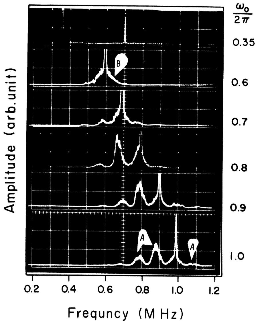
Fig.7 Frequency spectra of received wave signals at various  $\omega_0$ . Only lower amplitude parts of the spectra are shown in order to emphasize the sidebands.  $\omega_{pi}/2\pi = 1.3$  MHz.  $x = 5$  cm.  $V_{ex} = 1$  volt p-p.
