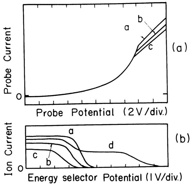
Fig.2 (a) Langmuir probe curves and (b) ion energy analyzer curves, when DC potential difference is applied between two plasmas. a;  $V_{ex} = 1$  volt, b;  $V_{ex} = 0$ , c;  $V_{ex} = -1$  volt, and d;  $V_{ex} = 5$  volts.
