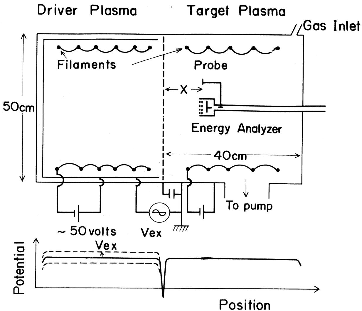
Fig.1 Layout of DP-machine. The potential profile is shown at the bottom.
