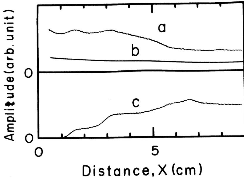
Fig.10 Amplitude of the carrier waves (a and b) and of the first lower sideband (c) as a function of distance.  $V_{ex} = 1$  volt for curve a and c.  $V_{ex} = 0.3$  volt for b. No sidebands grow in the case of curve c. Gain of the receiver is increased by 5 times for curve c.  $\omega_0/2\pi = 0.8$  MHz.  $\omega_{pi} = 1.1$  MHz.
