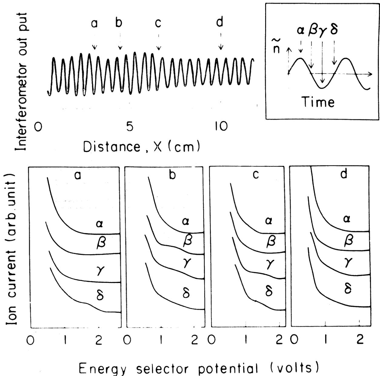
Fig.6 Ion energy analyzer curves at various positions (a, b, c and d), specified on the interferometer curve, and at various phase ( $\alpha$ ,  $\beta$ ,  $\gamma$  and  $\delta$ ) of the wave specified in upper right sub-diagram.  $\omega/2\pi = 0.5$  MHz.  $\omega_{pi}/2\pi = 1.2$  MHz.  $V_{ex} = 1.2$  volt p-p. The energy selector voltage ordinate, which is proportional to  $V^2$ , has the effect of making the bump on the distribution seem broader than it is.
