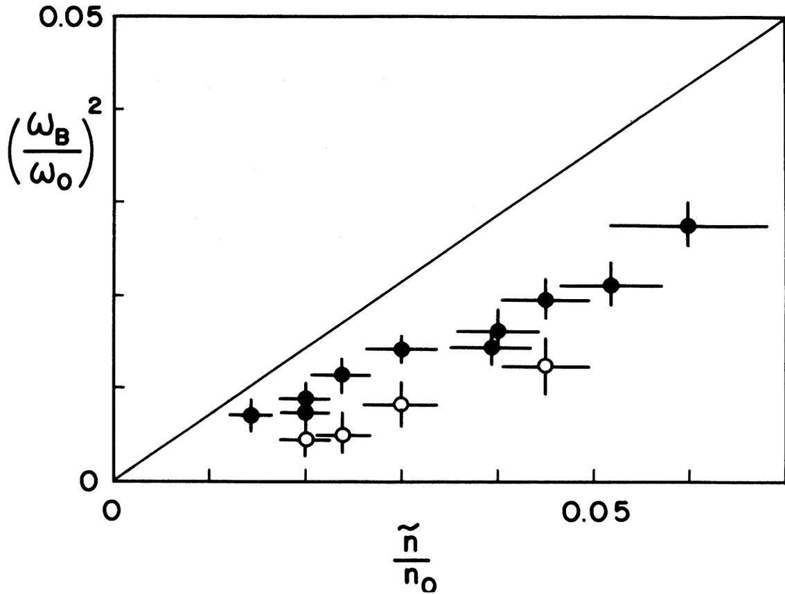
Fig.9 Bounce frequency as a function of wave amplitude. Solid line shows the relation  $(\omega_B/\omega_0)^2 = \sqrt{2} \tilde{n}/n_0$ . Dots are experimental points from the period of the amplitude oscillation. Open circles show  $\omega_B$  obtained from the frequency of the sideband via Eq.(1a) and the experimental dispersion curve.
