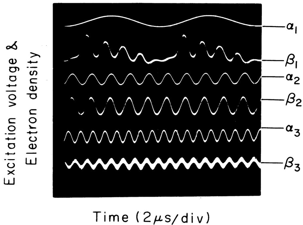
Fig.4 Excitation voltages  $V_{ex}$ , labeled by  $\alpha$  (2 volts/div.) and perturbed electron density  $\tilde{n}$ , labeled by  $\beta$  ( $\tilde{n}/n = 0.1/\text{div.}$ ), as a function of time. Excitation frequencies are 0.1 MHz for  $(\alpha_1, \beta_1)$ , 0.5 MHz for  $(\alpha_2, \beta_2)$  and 0.8 MHz for  $(\alpha_3, \beta_3)$ .  $\omega_{pi}/2\pi = 1.1$  MHz. Distance from the wave excitation point,  $x$ , is 7 cm.
