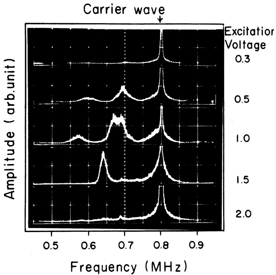
Fig.8 Frequency spectra of the sideband waves at various excitation voltage (peak to peak values are written).
