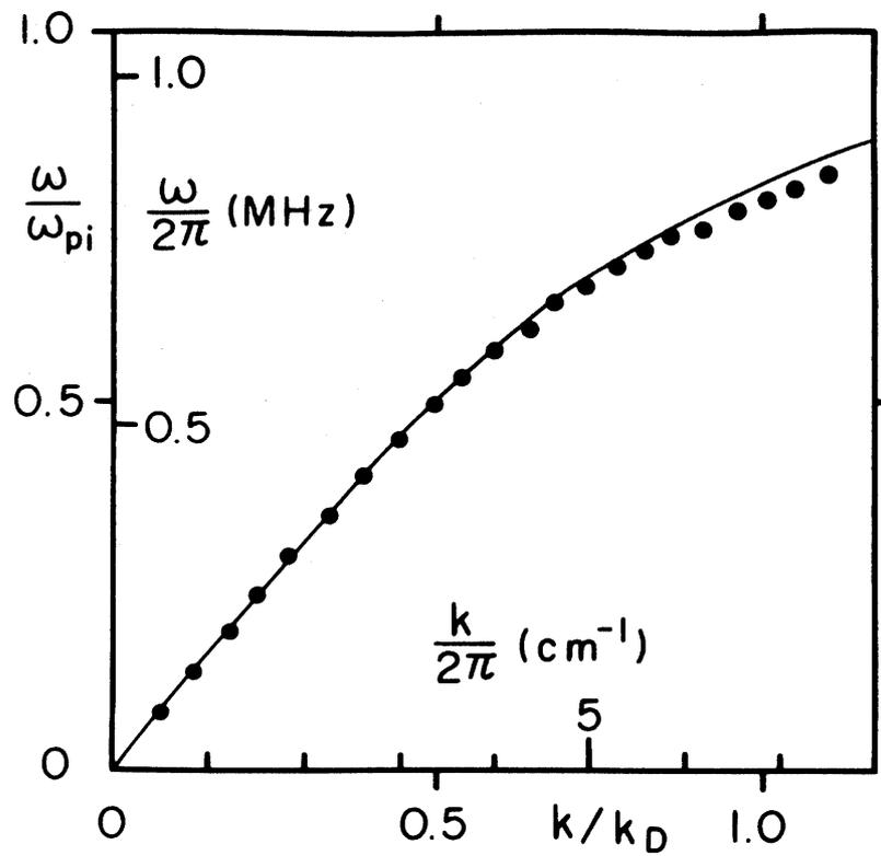
Fig.3 Dispersion relation of ion-acoustic waves. Dots are experimental points; curve shows Eq.(3) for  $T_e/T_i = 20$ .
