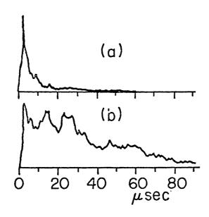
Fig.3. Typical waveforms of output signal from neutral particle analyzer; (a) without plasma current and (b) with plasma current. The particle energy is 600 eV.
