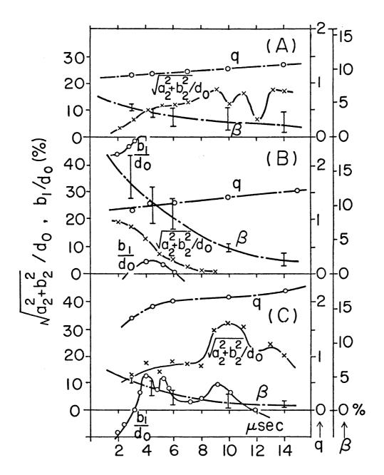
Fig.8. Typical examples of time evolution of q,  $\beta$ , amplitude of m = 2 mode  $(\sqrt{a_2^2 + b_2^2})/d_0$ ) and sine component of m = 1 mode  $(b_1/d_0)$ .
