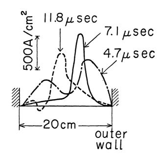
Fig.ll. The current distribution across the plasma, the operating condition is the same as that of Fig.9 but without vertical field.
