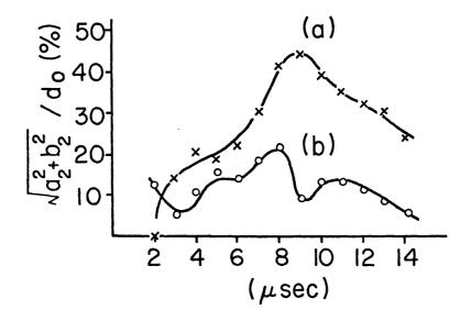
Fig.10. The time evolution of the amplitude of m=2 mode under the operating condition of Fig.9; (a) without vertical field and (b) with vertical field.
