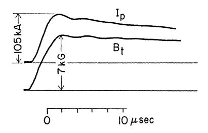
Fig.2. Typical waveforms of plasma current  $\mathbf{I}_{\mathbf{p}}$  and main toroidal magnetic field.
