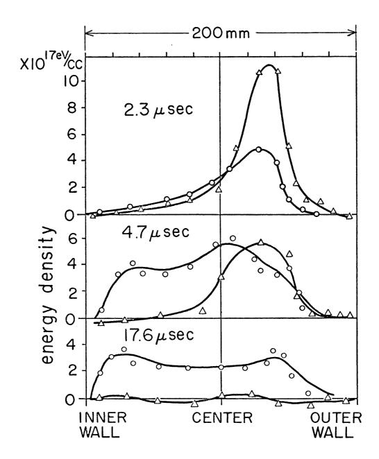
Fig. 9. The time evolution of pressure distribution with and without vertical field. Here, max.  $B_{t}$  is 9 kG and max.  $I_{p}$  is 85 kA. Circles, with vertical field; triangles, without vertical field.
