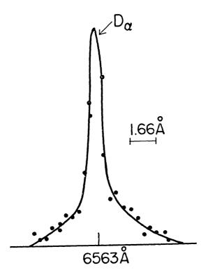
Fig.4. A typical Doppler profile of  $\textbf{D}_{\alpha}$  line.
