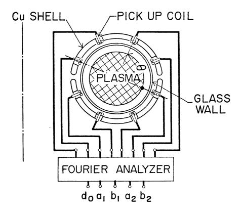
Fig.6. A schematic drawing of the system of eight magnetic probes around the discharge tube. Signals from magnetic probes are converted into five Fourier components using the relation,
