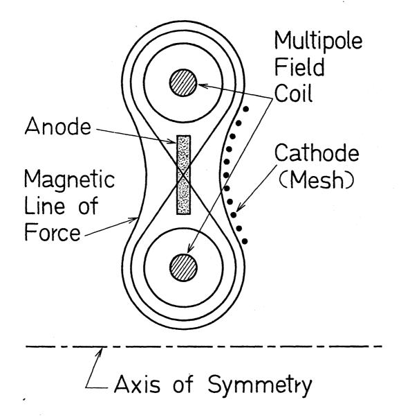
Figure 1. A design of the possible ion beam source.
