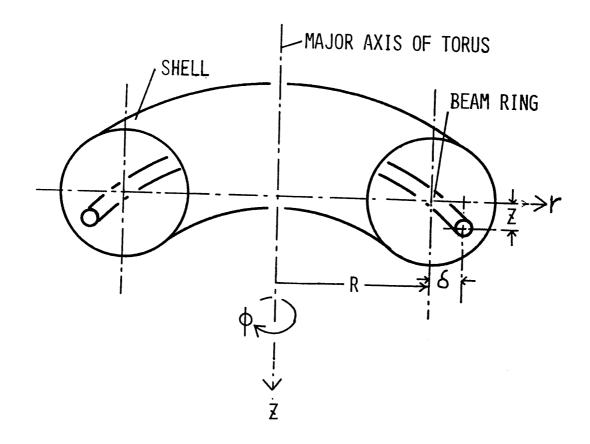
Fig.1 Cross-section of torus showing the coordinates  $(r, \phi, z)$  and the position of the beam ring.
