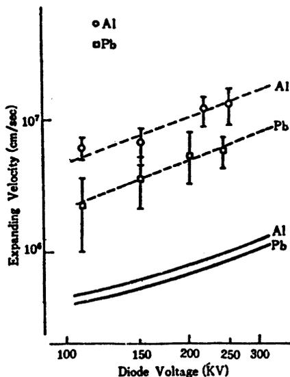
Fig. 2 Ion velocity measured by time of flight method
