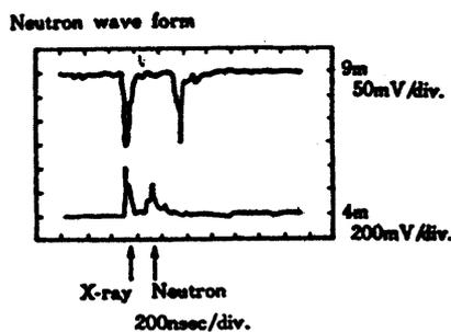
Fig. 3 Neutron signal on plastic scintillation counter
