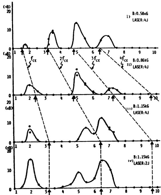
FIG. 4. Frequency spectra of the long-lasting microwave emissions (emission C);  $B$  is the external magnetic field strength and LASER means the laser energy for the production of the plasma. Electron cyclotron harmonics are denoted by arrows in each spectrum.
