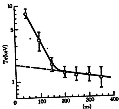
Fig. 1 Electron temperature of plasma as a function of time
