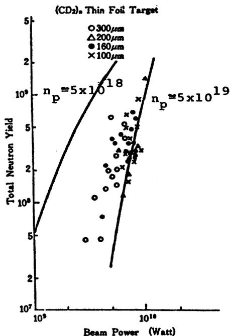
Fig. 4 Dependence of neutron yield on beam power for the CD<sub>2</sub> target of various thickness and estimated value ( solid line ).
