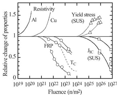
**Fig. 1** Neutron-induced deterioration of a superconducting magnet element. Electric resistance, mechanical strength,  $T_c$ , and a yield stress and  $J_c$  are selected as indexes of properties for stabilization material, insulator (FRP), superconducting material, and SUS, respectively.
