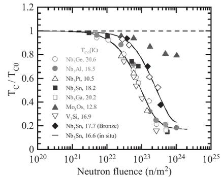
**Fig. 2** Degradation behavior of  $T_c$  of compound-system superconductor.
