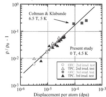
**Fig. 3** 14MeV neutron irradiation effect on electric resistance.
