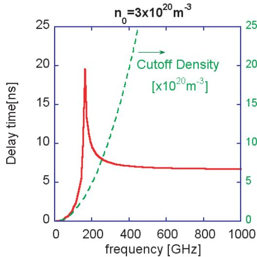
Fig. 2 Delay time of the launched THz wave as a function of frequency. Here, the estimated density profile is the same in Fig. 1.
