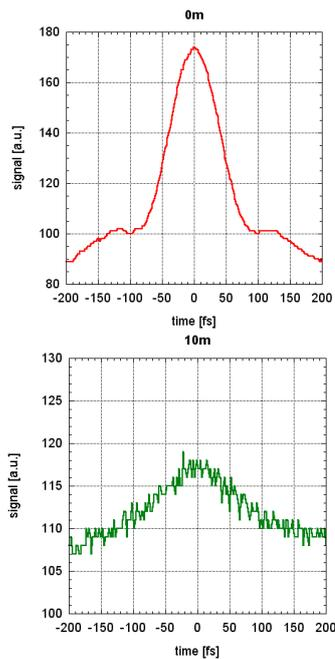
Fig. 7 Waveform of auto-correlated signal w/o fiber (top) and with 10 m fiber (bottom).
