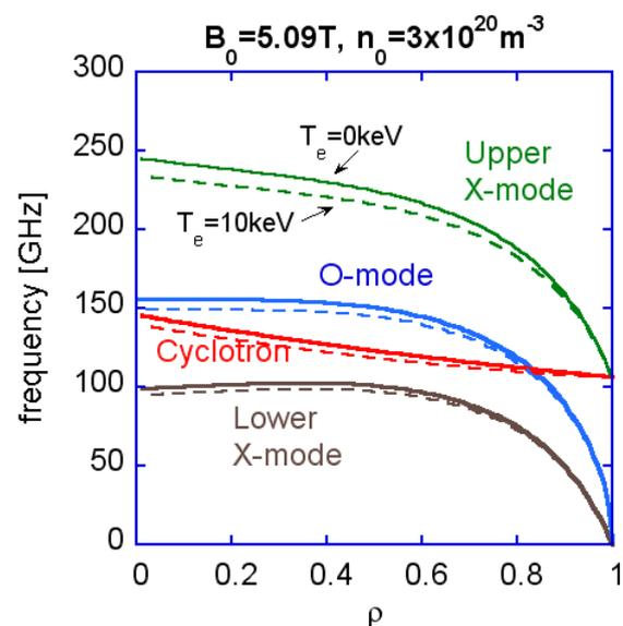
Fig. 1 Radial profile of characteristic frequencies in a typical plasma parameter of helical DEMO. “O-mode” means ordinary wave cut-off frequency that is the electron plasma frequency. “Cyclotron” means the electron cyclotron frequency. “Upper and Lower X-mode” mean the right-hand and left-hand extraordinary wave cut-off frequencies. Dotted line includes the higher temperature effect (relativistic effect).
