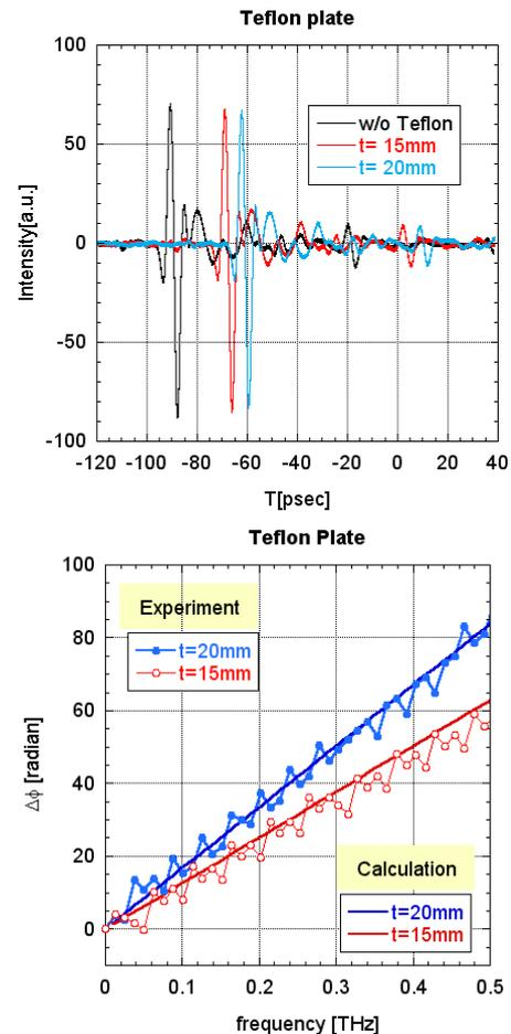
Fig. 6 Waveform of THz pulse penetrating through the Teflon plate (upper). The phase difference ( $\Delta\phi$ ) as a function of the frequency (bottom).
