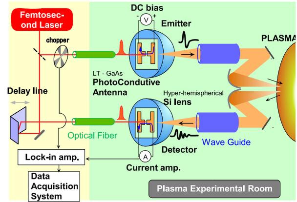
Fig. 3 Schematic drawing of THz reflectometer/delayometer system.
