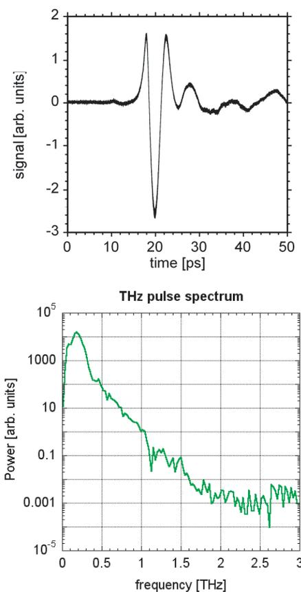
Fig. 5 Detector output signal (upper) and its frequency spectrum (bottom).
