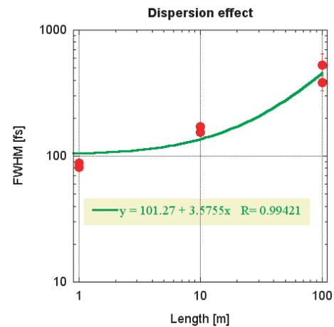
Fig. 8 Pulse width via the optical fiber which lengths are 1, 10, and 100 m.
