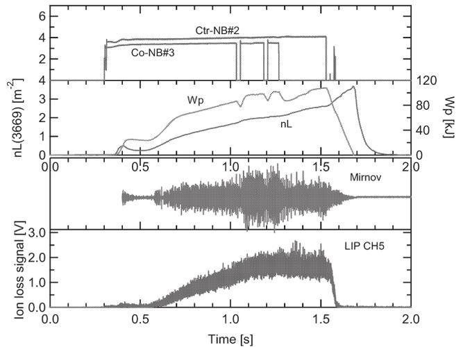
Fig. 2. Fast ion loss signal and magnetic probe signal. The fast ion loss corresponds to the pitch angle of around 130 degrees.
