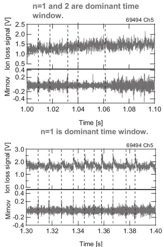
Fig. 3. Fast ion loss signals with unclear and clear bursts.
