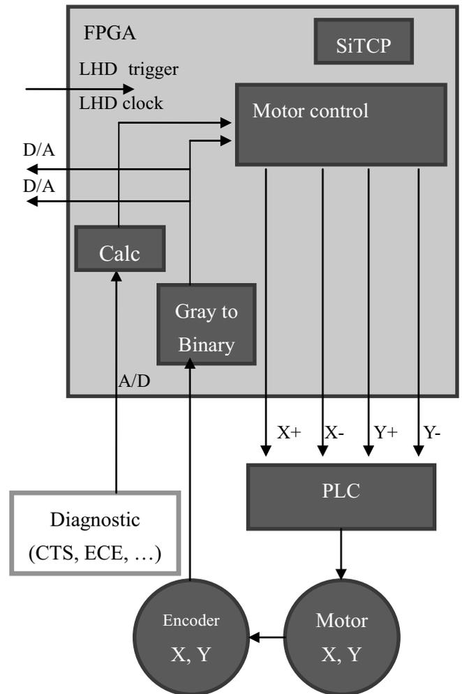
Fig. 2 Conceptual diagram of antenna feedback system for ECH/ECCD.
