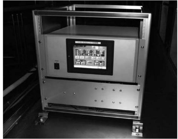
Fig. 1 PLC based control system for the 1.5L-ECH antenna.
