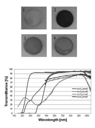
Fig.1 Transmittance of samples SOC-1, 2, 3, and 4 after JRR-3 irradiation (48 hours, 22K2009).
