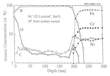
Fig. 1 Depth profile obtained with the in-situ AES analysis.
