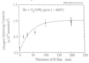
Fig. 2 Oxygen gettering capacity as a function of B-film thickness.
