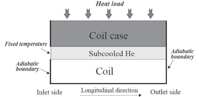
Fig. 1. Analytical model of the LHD helical.
