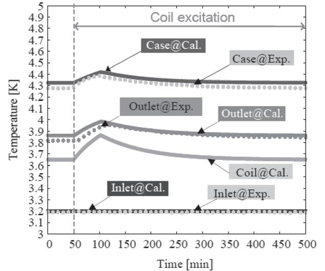
Fig. 2. Temperature profiles in the experiment and calculation under coil excitation from 0 A to 13 kA with the ramp rate of 3.5 A/s. During the coil excitation, the inlet temperature of 3.2 K and the mass flow of 50g/s were kept.
