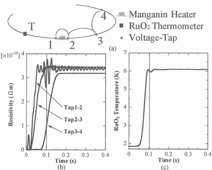
Fig. 1. Positions of measuring elements, and measured waveforms of resistivity and temperature
