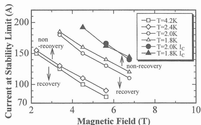
Fig. 2. Stability limits for test coil for 73 mJ heat input
