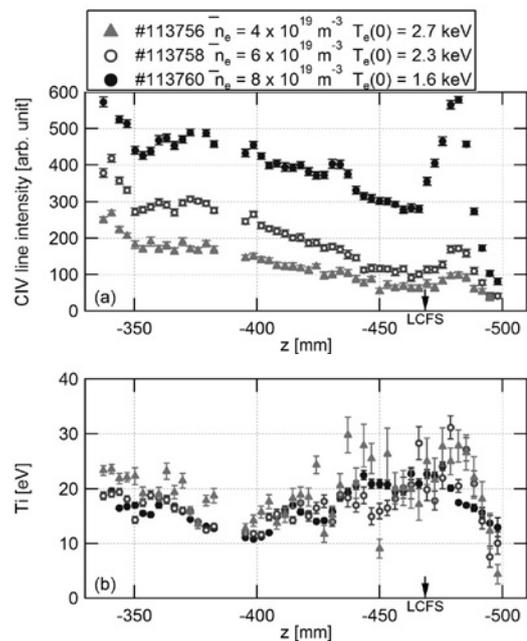
Fig. 2. Vertical profiles of (a) CIV line intensity and (b) ion temperature derived from the Doppler broadening of CIV spectrum.
