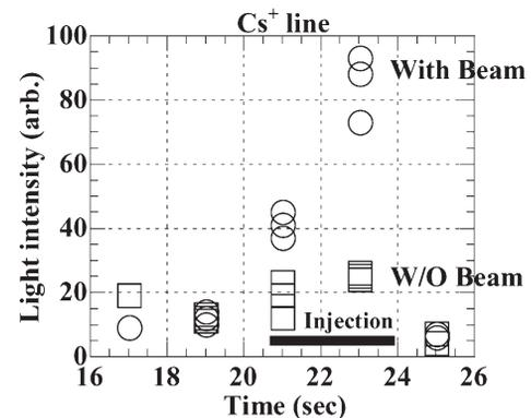
Fig.3 Temporal dependence of CsII(Cs<sup>+</sup>) line intensity with- or without beam acceleration voltage.
