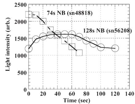
Fig. 1 Temporal dependence of H<sup>-</sup> production during long-pulse injection. With an actively cooled PG in 128s injection. With a little conduction cooling PG in 74s one.
