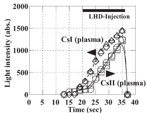
Fig.2 Temporal dependence of CsI(Cs<sup>0</sup>) and CsII(Cs<sup>+</sup>) line intensity from plasma source during the NB injection.
