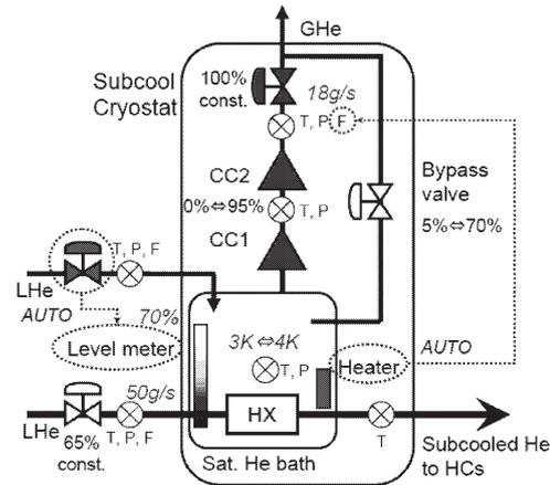
Fig. 1 Schematic diagram of the control equipments.
