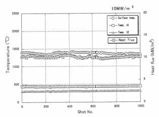
Fig.3 Relationship between the temperatures of a mock-up and the shot number of a cyclic heat load of  $10 \text{ MW/m}^2$ .
