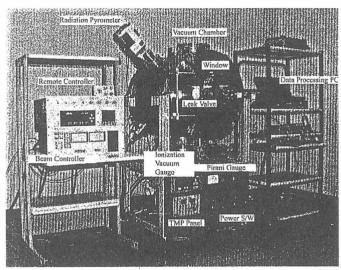
Fig. 1 Deflection-type electron beam heating apparatus.
