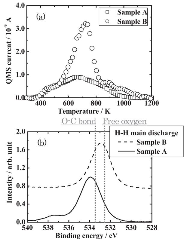
Fig. 1 (a) The H<sub>2</sub> TDS spectra and (b) the O-1s XPS spectra for the boron samples deposited in LHD and by P-CVD after H-H discharge exposure.
