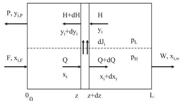
Fig. 2 Schematic view of membrane module in counter-flow model
