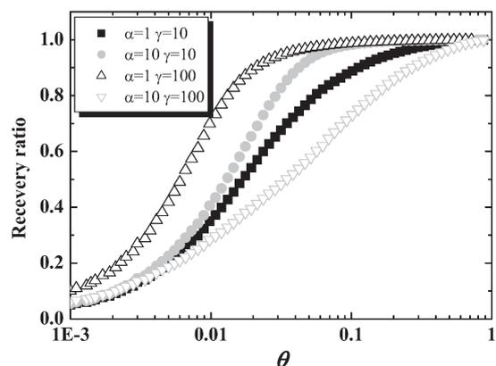
Fig. 3 Simulation results of counter-flow model as a function of separation coefficient
