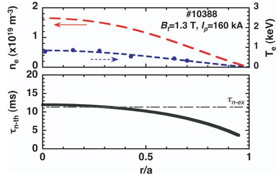
Fig. 3 Radial profiles of the electron density,  $n_e$ , and the temperature,  $T_e$  (top) in the discharge at  $B_t/I_p$  of 1.3 T and 160 kA and the D-D neutron decay time,  $\tau_{n-th}$ , predicted by the classical slowing-down model. The experimentally evaluated neutron decay time,  $\tau_{n-ex}$ , is also drawn.
