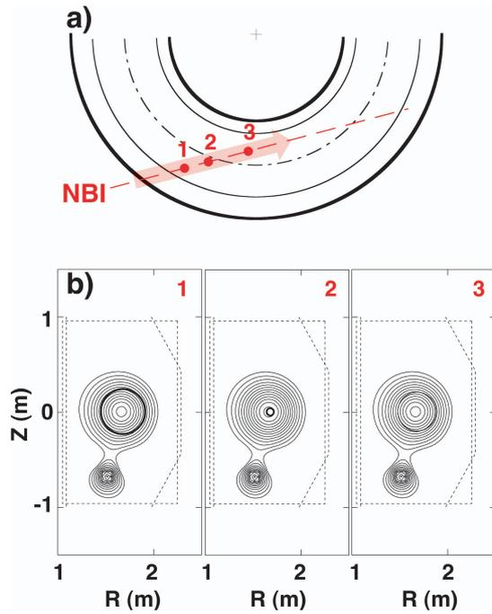
Fig. 1 a) Arrangement of the NBI on the HL-2A.  $B_t$  and  $I_p$  are oriented to be CW and CCW, respectively, as seen from the top. b) Initial collisionless orbits of beam ions with  $E$  of 30 keV on the center of the beam line at plasma of  $B_t = 2.4$  T/ $I_p = 305$  kA and  $q_{95}$  of  $\sim 3.8$ .
