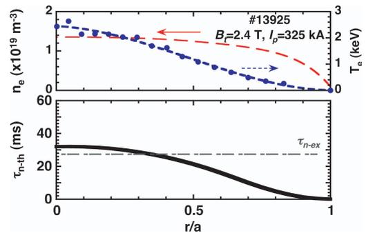
Fig. 4 Radial profiles of the electron density,  $n_e$ , and the temperature,  $T_e$  (top) in the discharge at  $B_t/I_p$  of 2.4 T and 325 kA and the D-D neutron decay time,  $\tau_{n-th}$ , predicted by the classical slowing-down model. The experimentally evaluated neutron decay time,  $\tau_{n-ex}$ , is also drawn.
