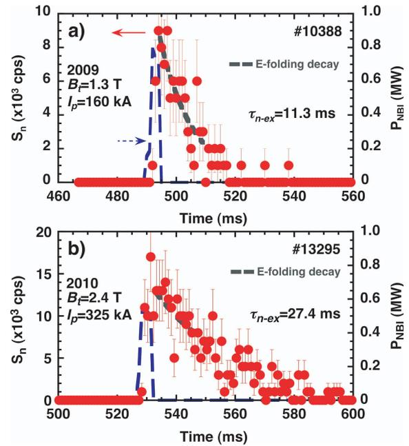
Fig. 2 a) Time evolution of the neutron emission rate  $S_n$ , when the deuterium beam blip is injected into the MHD quiescent ohmic plasma in  $B_t/I_p$  of 1.3 T/160 kA. b) The neutron emission rate due to the beam blip in  $B_t/I_p$  of 2.4 T/325 kA. The line-averaged electron density ( $\sim 1 \times 10^{19} \text{ m}^{-3}$ ) and  $q_{95}$  ( $\sim 3.8$ ) are kept for both plasmas.
