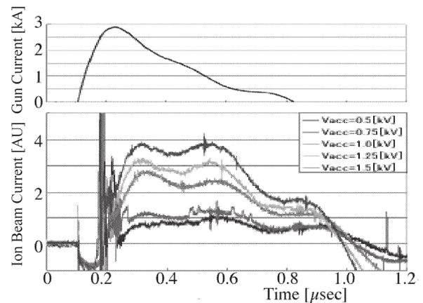
Fig. 2 Time evolutions of the washer gun current and ion beam currents measured by Faraday cup under five different voltages applied to the acceleration electrode.
