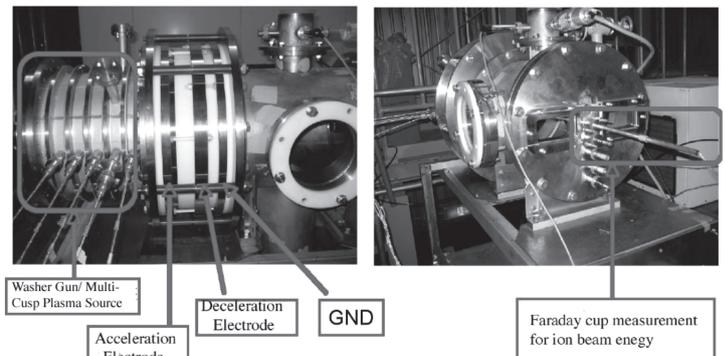
Fig. 1 Low-voltage/ high-current NBI device with washer gun, where new electrode system was installed.
