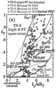
Fig. 2(a)  $\beta_T$  of the single ST (no merging) and high-beta STs produced by merging (a) and (b) as a function of  $I/aB_t$ ,
