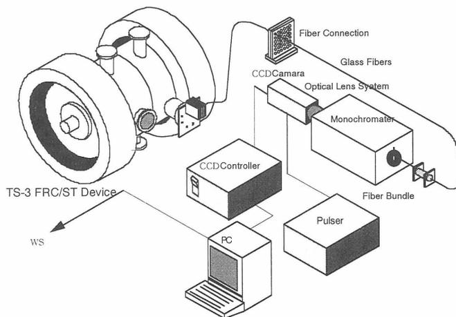
Fig. 1. Visible light tomography system and its tentative set-up at University of Tokyo.
